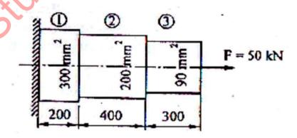
**Q.4** Figure below shows the bar with dimensions and loads. Determine the nodal displacements, element stresses, if the temperature rises by 60 °C. Assume the modules of elasticity for the complete bar as 200 GPa and coefficient thermal expansion as 12 x 10<sup>-6</sup> per °C.
